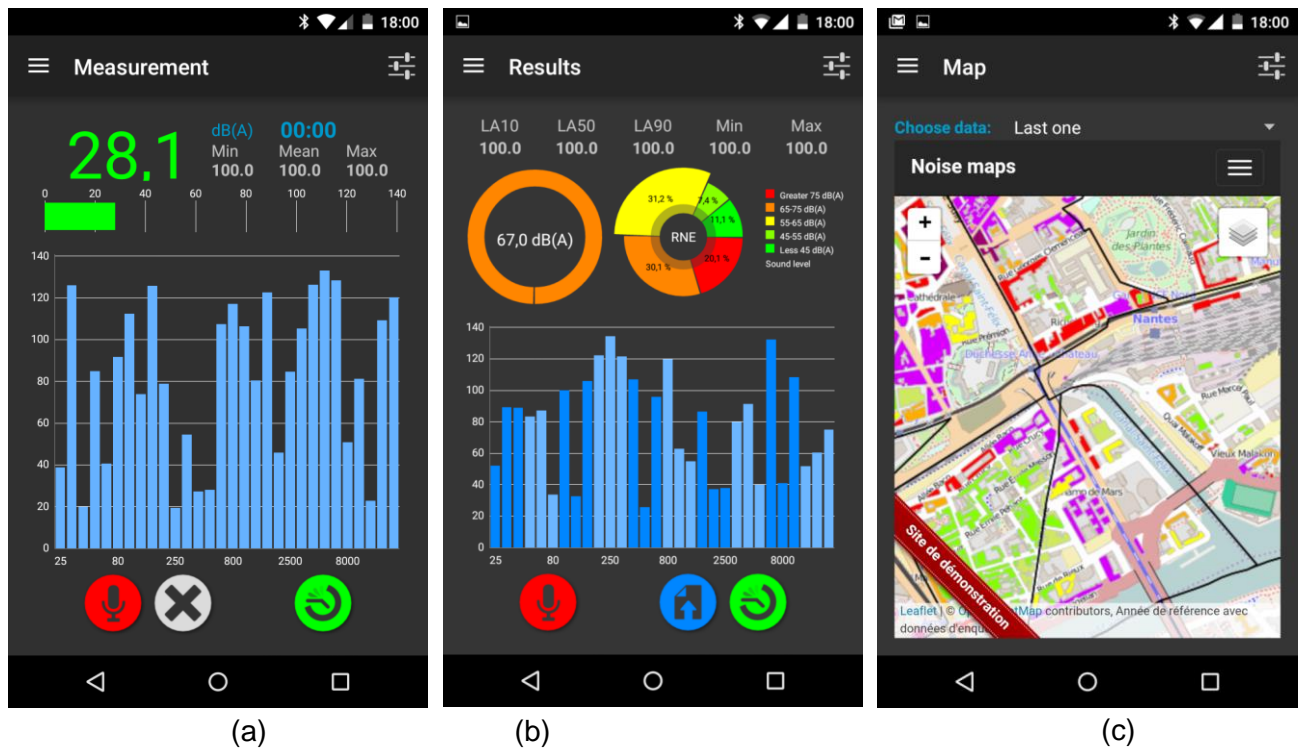
Figure 15: Screenshots of the NoiseCapture application: (a) measurement screen, (b) results screen and (c) noise map visualization
